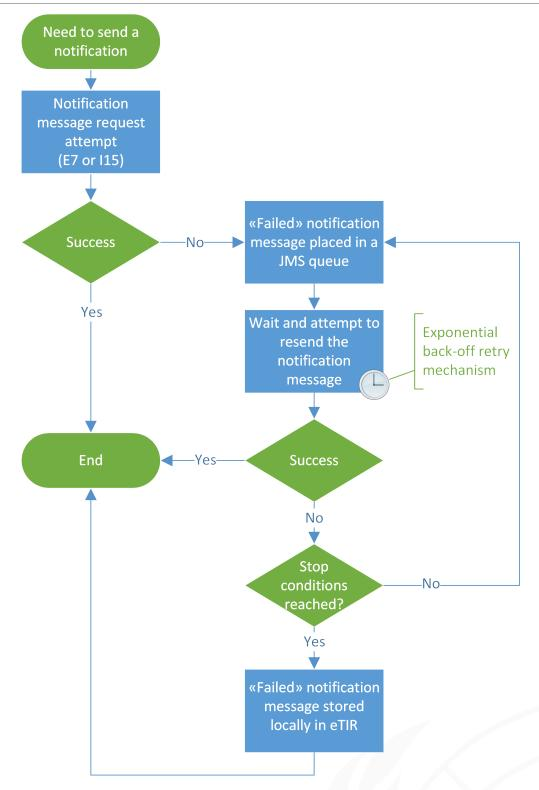
This mechanism relies on the **exponential back-off retry algorithm** allowing for progressively longer delays when retrying attempts in order to increase chances of success.
