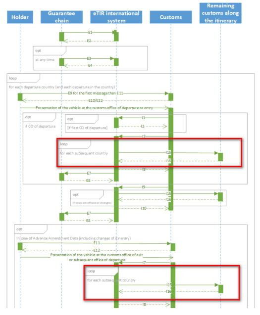
When a customs office of departure (the first one or a subsequent loading point) sends the I7 - Record declaration data message, the eTIR international system forwards this declaration data to the remaining countries along the itinerary.
