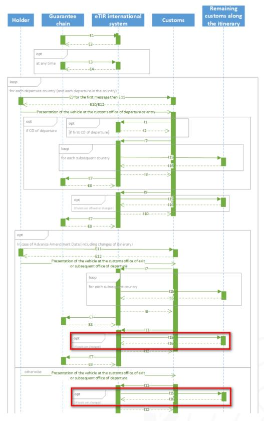
When seals are changed, following an inspection, when terminating a TIR operation, the eTIR international system forwards the information about the new seals to the remaining countries along the itinerary.
