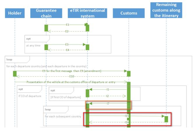
The eTIR international system uses a queuing system to retry sending notifications. The diagram below illustrates this fallback mechanism:
