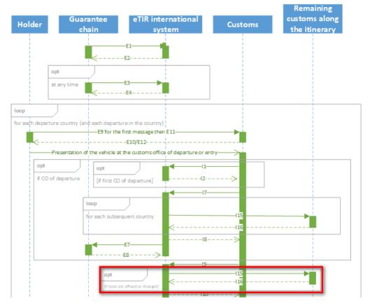
When seals are affixed for the first time at the initial customs office of departure or when seals are changed, following an inspection, when starting a TIR operation, the eTIR international system forwards the information about the new seals to the remaining countries along the itinerary.
