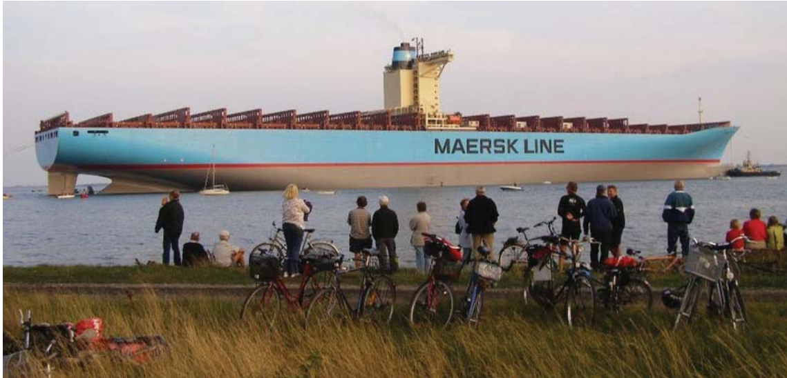
The world's biggest container ship Emma Mærsk is fitted with the largest diesel engine ever manufactured (110,000 hp). She beats all former containerships by 10 per cent. The ship can carry 13,000 containers all over the world.
